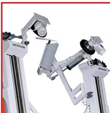
This is a steel frame made of two struts connected to each other by a base so as it can be easily detached. The sturdy properties of this frame enable the lifting of bowl-trolleys with capacities from 120 to 300 kg).
